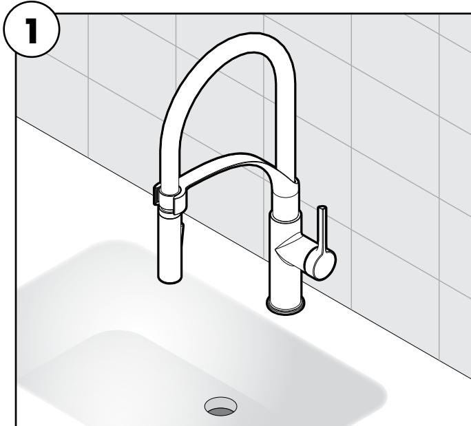
Fits 1-hole sink (without using deck plate (C) and putty plate (D)).
